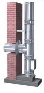
MKDZ The bold-insulated double-wall system used as a standalone external chimney for solid fuel fired boilers. It allows for setting the heating unit anywhere in the facility. The chimney is carried outside and mounted on the wall. It comes in version: Premium for coal, wood, pellets, pea coal. The system can operate only in dry working conditions at temperatures up to 600°C
