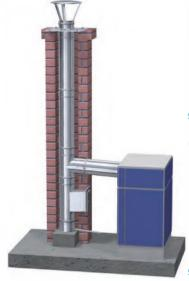
MKS The single-wall system used as a liner for open combustion chamber boilers or as connection elements for insulated chimneys. This allows for the modernization of boiler houses and adaptation of old chimney to the new working conditions. It comes in two versions: Premium for gas, oil, wood, pellets. Standard for boilers working on gas and oil. The system can operate only in dry working conditions at temperatures up to 450°C. It is also available in oval and rectangular version.
